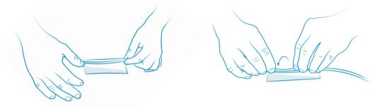
Maintaining close contact between the plastic film and the latex tubing, roll the latex tube forward until it is completely wrapped with the plastic film. Roll the assembly a few times so that the plastic film fits snugly to the latex tubing.
